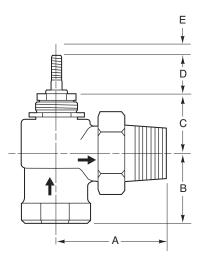
Figure-5 Dimensions for VB-7211-0-3-P Series Angle Valve Bodies.
