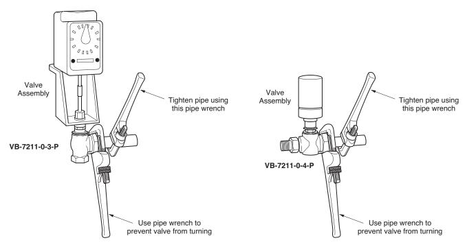
Figure-4 Installation of Union End Valves.
