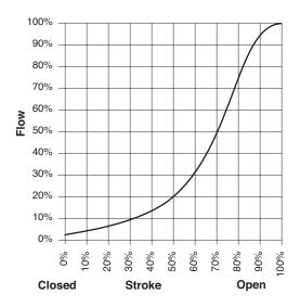
Figure-1 Typical Modified Equal Percentage Flow Characteristics.
